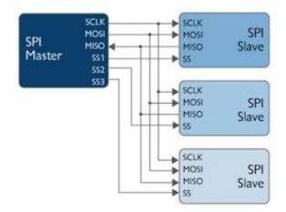
SPI wiring master to three slave devices
