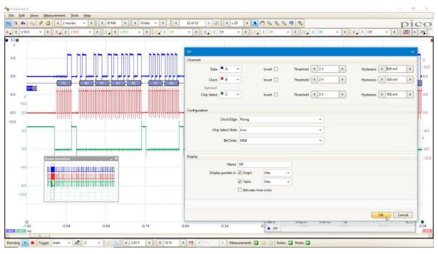
In the SPI configuration menu, check both the In Graph and the **In Table** boxes to display SPI packets correlated in time with the acquired data channels plus a tabular listing of the packets. Double-click a packet in the graph view to see the same packet in the table view, and vice versa.
