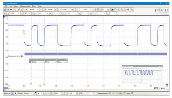
Manchester encoding uses an exclusive-OR Boolean function to combine the clock and data on a single channel. This means that binary information is conveyed as transitions rather than levels.
