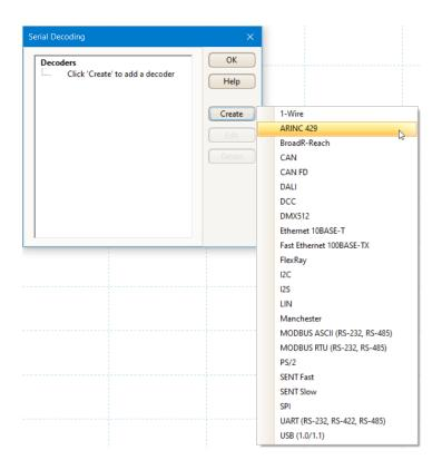
In the ARINC 429 configuration menu select the appropriate PicoScope input channel, baud rate and any other parameters as necessary. Click **OK** to see the decoded ARINC 429 messages in the PicoScope graph display.
