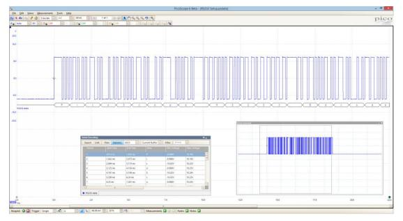
The PicoScope RS-232 decoder can also handle similar serial data standards such as RS-422 and RS-485  $\,$
