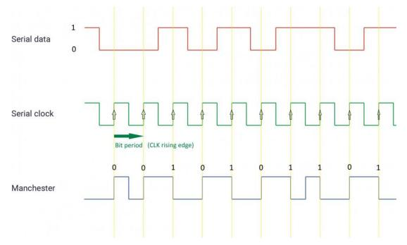
As with any engineering design choice, these advantages don't come for free. Embedding the clock doubles the required network bandwidth. But for many applications Manchester is a good and widely used communications protocol.
