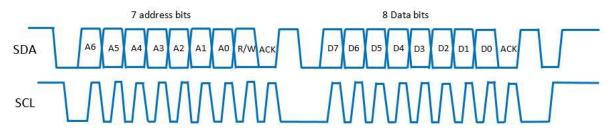
At the start of packet a master device takes control of the bus by driving SDA low while SCL remains high. This indicates that a message will follow.
