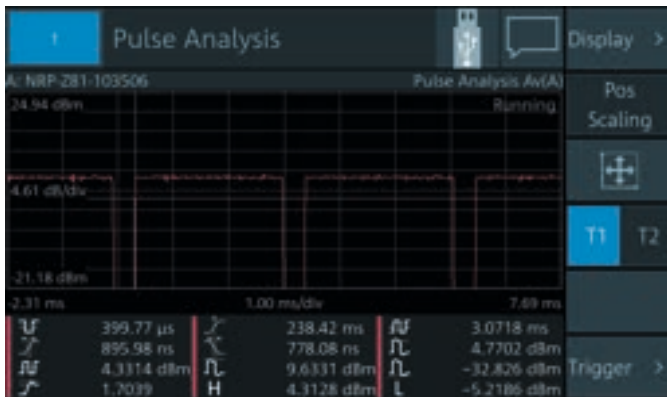
Automatic pulse analysis with the R&S®NRX and R&S®NRP-Z81
