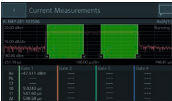
Determination of power of an EDGE burst using an R&S®NRPxxS(N) three-path diode power sensor and the gate function; exclusion of training sequence in the center of the signal
